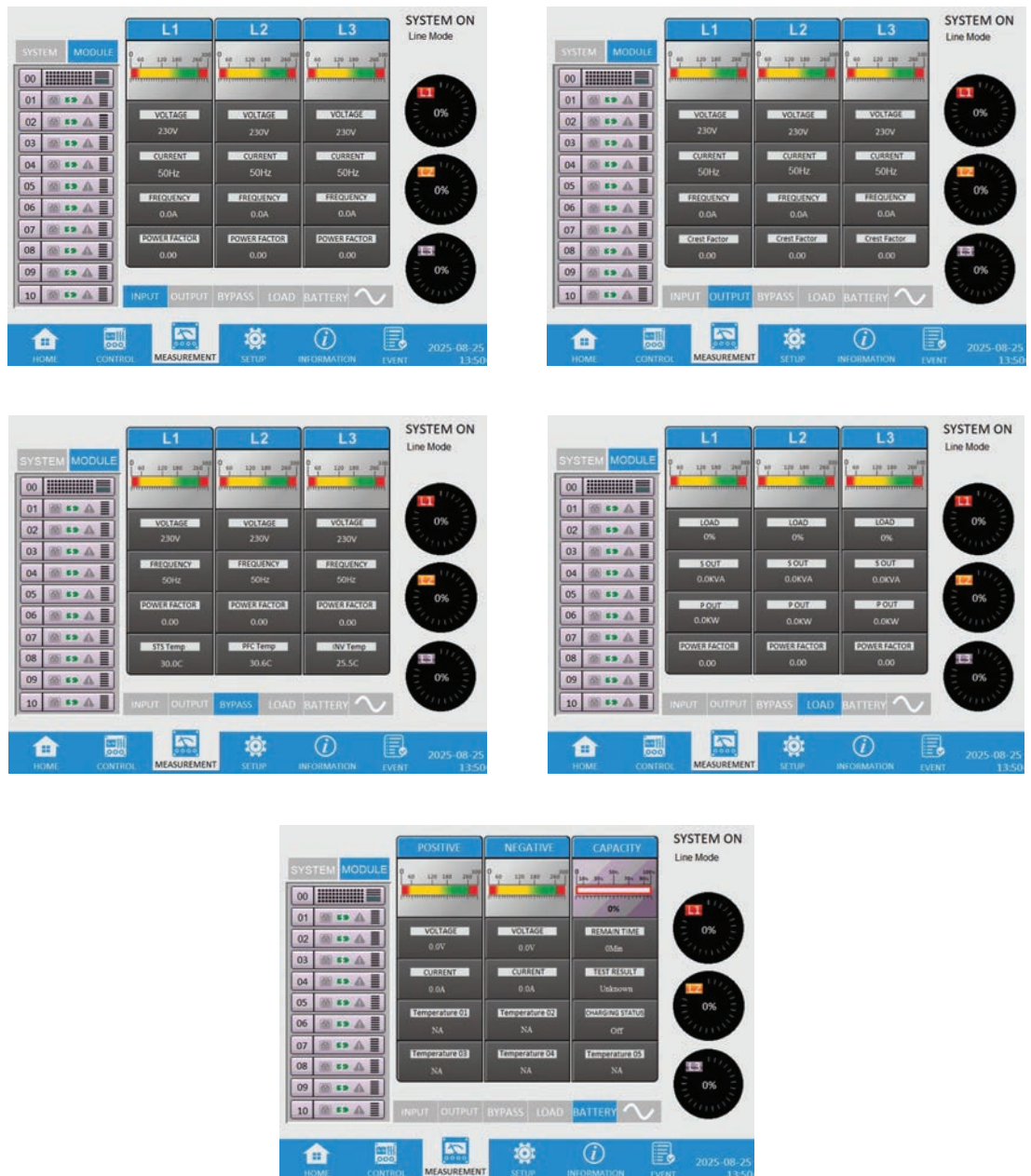
Figure 4-10 Module Measurement Screens
