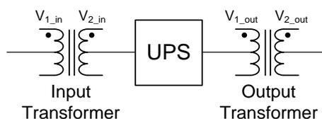
$$\text{Input transformer ratio} = V_{1\_in}/V_{2\_in} = T60$$
