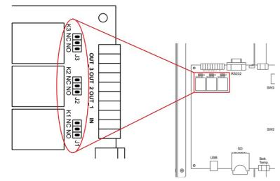
Short/circuit the input contact to send a command to the UPS.
