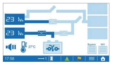
6- Close the battery breakers only after the rectifier has been turned on.
