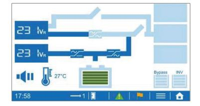
7- The inverter will be started and supply output voltage.
