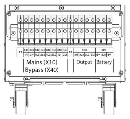
If the UPS is installed in a TN-C system, it is necessary to connect together the input, bypass and output neutral on the terminals during the installation as shown in the following picture. For the connecting cable between X40-2N and X50-3N, use a cable with a maximum cross section of 10 mm<sup>2</sup> to be terminated together with the neutral cable with a tube terminal.
