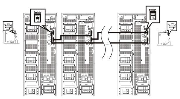
The parallel communications cable must be plugged as shown below.
