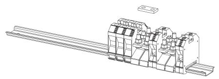
4. Separate the positive terminals +0 and +1 and insert the insulating functional separator supplied in the accessory kit into the DIN rail.
