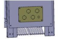
In the case of the Trimod HE 80 kVA, the cables must be passed into the opening at the base. The fastening is done on the appropriate bar by means of clamps and clips present in one of the accessory packs.
