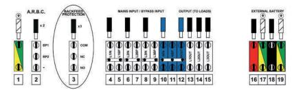
If the UPS detects a voltage backfeed, the relay is energised and changes status, enabling the disconnection of the input lines that must be done externally as indicated in the diagrams shown below. The relay contacts characteristics are :
