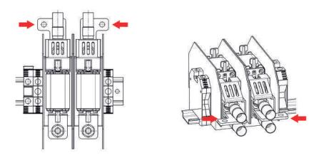
4.2.7.1 Connection of one external modular battery cabinet to the Trimod HE 10-15-20-30TT/TM
