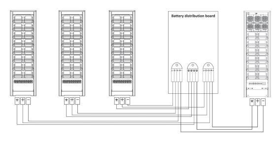
The external modular battery cabinets must be connected to the switchboard with the multipolar cables provided. The external non modular battery cabinets must be connected with external cables according to the instructions given in table 8 of chapter 10.
