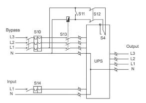
Single phase/Three phase configuration (available only for SINGLE PHASE input and THREE INDEPENDENT PHASES output)
