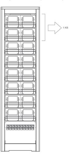
It is necessary to install 1 KB every 10 kVA of nominal UPS power in case of modular cabinets with battery drawers. For example, for the Trimod HE 40 TT it is necessary to have at least one external modular battery cabinet with 4 KB (16 battery drawers).
