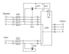
Single phase/Three phase configuration (available only for SINGLE PHASE input and THREE INDEPENDENT PHASES output)
