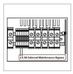
If External Maintenance Bypass would be used; connect normally open auxiliary contact of External Maintenance Bypass MCCB on the distribution panel to terminals **a/X6** and **b/X6** on UPS.
