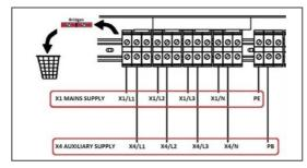
Connect the phase cables to X1 MAINS SUPPLY: X1/L1 - X1/L2 -X1/L3 terminals, the neutral to X1 MAINS SUPPLY: X1/N terminal.
