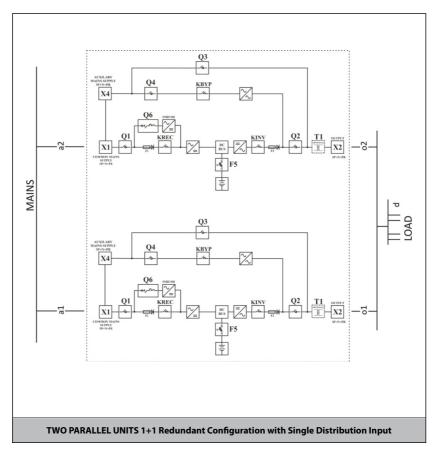
a1, a2: Mains Supply MCCB 4pd: Distribution MCCBo1, o2, unit output switch 4p
