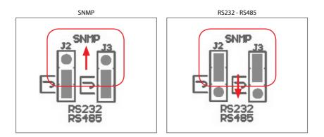
NMP JUMPER (J2 - J3): If internal SNMP would be used, 2 jumpers should be moved to upper side.
