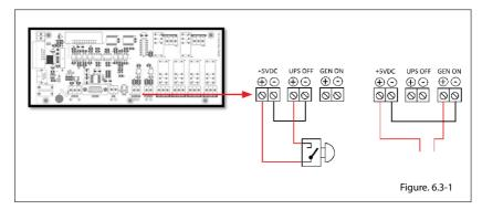
UPS output can be switched off immediately by Remote Emergency Switching Device interface (ESD) connection if desired. A remote latched switch can be used as described in above figure.
