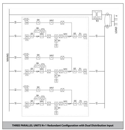
a1, a2, a3: Mains Supply MCCB 4p b1, b2, b3: Auxiliary Supply MCCB 4p
