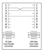
If Serial Communication cable is needed, it can be produced according to the pin configuration described at side.
