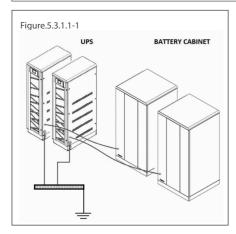
Input Mains Supply's Protective Earth terminal **PE** of the UPS shall be connected to the ground with a low impedance connection.
