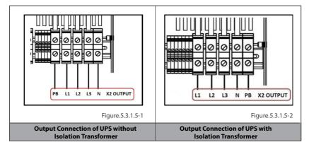
Connect the phase cable to **X2 OUTPUT: X2/L1 – X2/L2 – X2/L3** terminal and the neutral cable to **X2 OUTPUT: X2/N** terminal.
