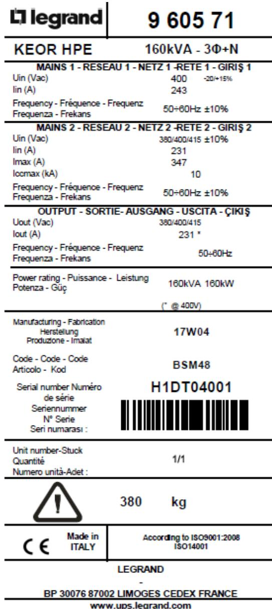
Picture 1 – Rating plate of KEOR HPE 60÷160 kVA
